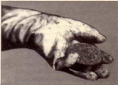
Plutonium metal puck. Plutonium is handled and stored in small quantities like this to prevent it from spontaneously starting a nuclear chain reaction. Photo courtesy DOE.
